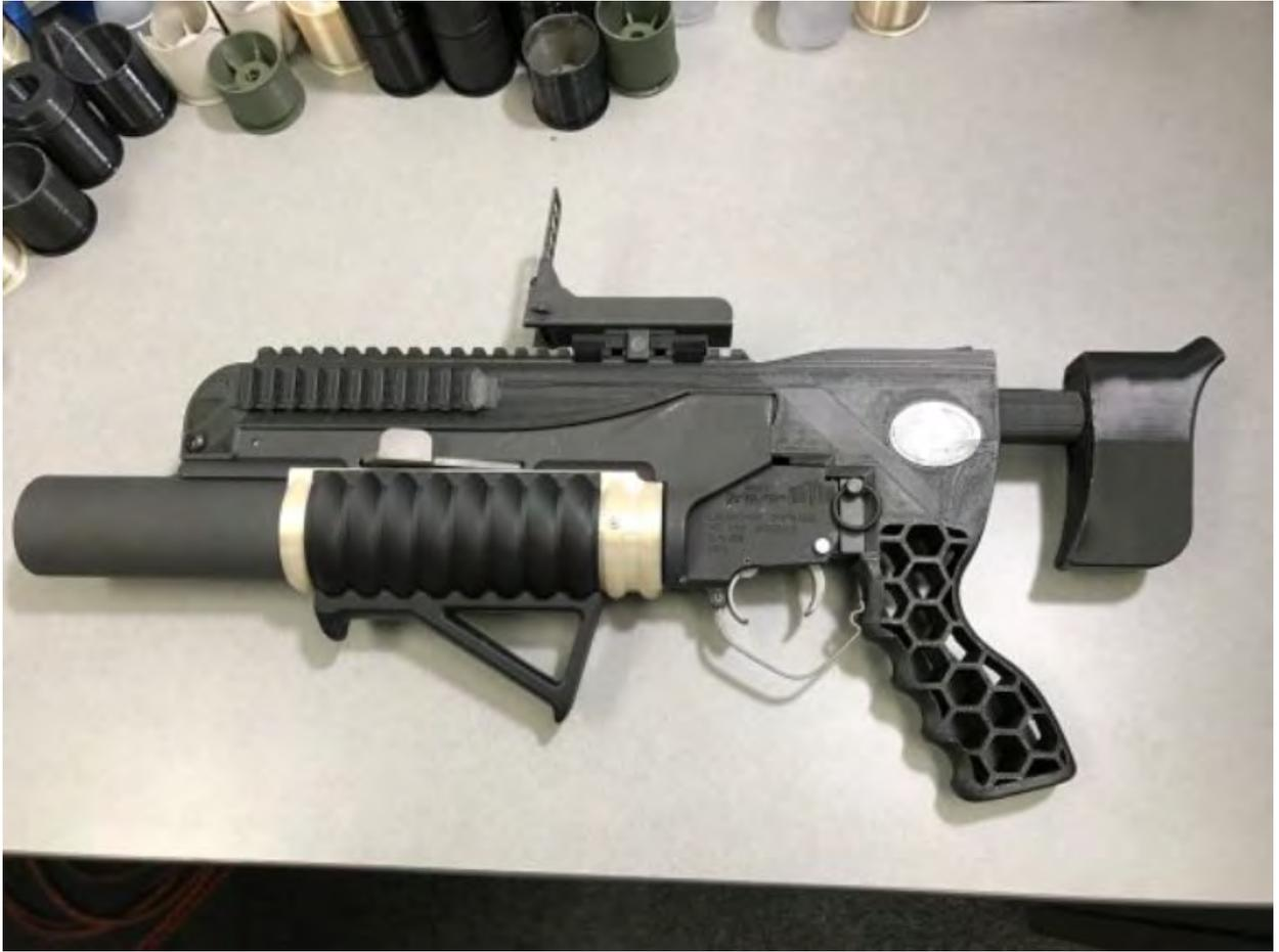
RAMBO took six months and was a teaming arrangement between the US Army Manufacturing Technology (MANTECH), US Army Research, Development and Engineering Command and America Makes. The purpose was to prove a complete weapon system could be additively manufactured to rugged enough to meet military standards.
