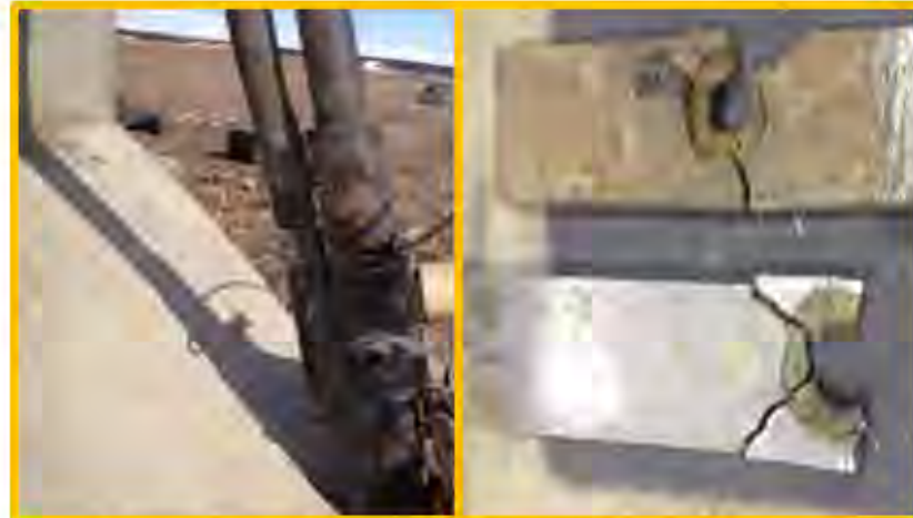
Charge placed on DshK using integral magnets Charge defeated 1" hardened steel.
