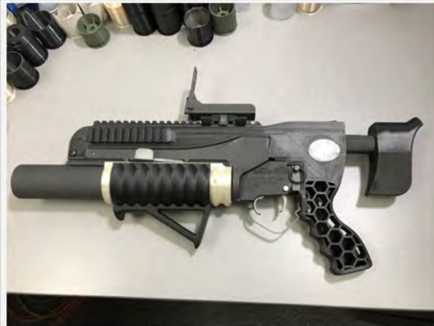
The additively-manufactured RAMBO system includes an NSRDEC-designed standalone kit with printed adjustable buttstock, mounts, grips and other modifications—modifications made possible by the quick turnaround time afforded by 3D printing.
