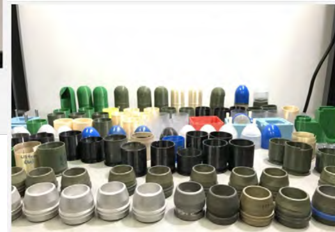
These M781 components were 3D-printed during a six-month collaborative effort that involved RDECOM, ManTech and America Makes, the national accelerator for additive manufacturing and 3D printing. They cost tens of thousands of dollars less than identical components created with standard production methods.
