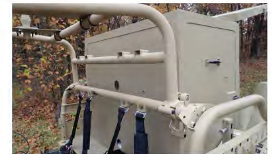
Rear of Enclosure showing Cabling Holes
