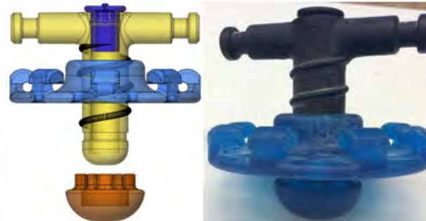
Screw type junctional tourniquet CAD (L), 3D printed assembly (R)
